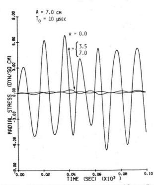
Fig. 8. Sound pressure generated in a sphere of 7-cm radius that simulates a human adult's head exposed to 918-MHz radiation.
