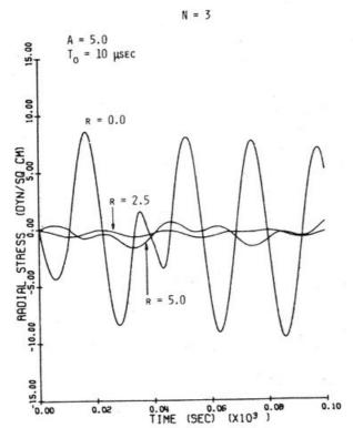
Fig. 6. Sound pressure generated in a sphere of 5-cm radius that simulates a human infant's head exposed to 918-MHz radiation.
